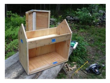
The roof's end trim pieces fit snugly outside the walls. Cut the 2"x2" brace for the roof so it fits snugly i nside the walls.
