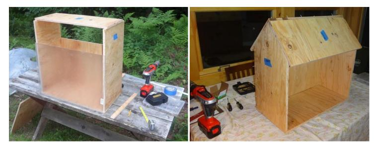
Follow your plan and revise it as needed. Measure and cut the walls, floor, and roof boards. To save problems later, be sure all cuts are square. Label each piece--otherwise it's easy to get a piece out of place. Trust me on this.
